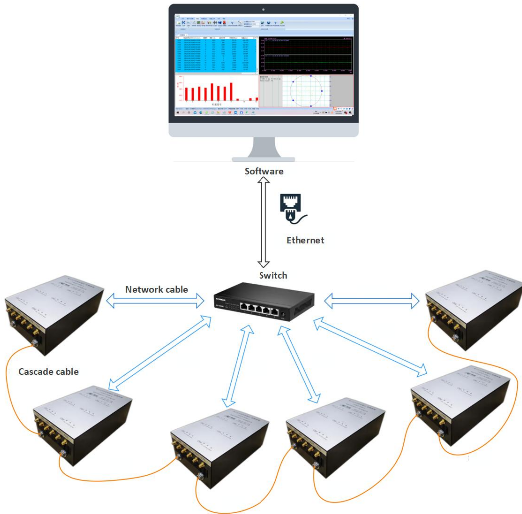
Fig. 2-2 Network connection of a RAEM1-6 desktop monitor
