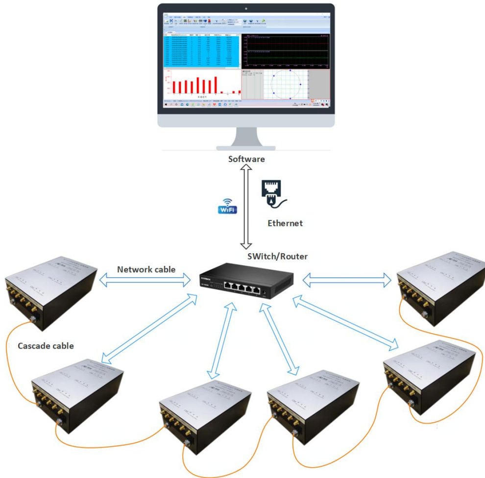
Fig. 2-7 Wi-Fi networking for RAEM1-6 desktop monitor
