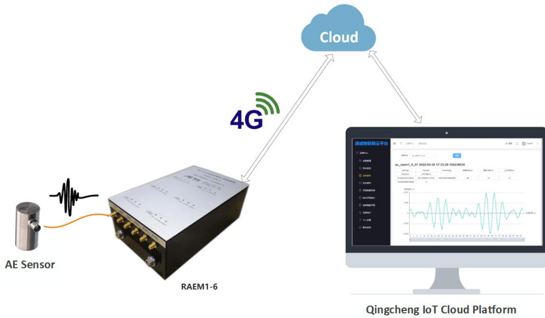
Fig. 3-2 RAEM1-6 Connecting to the cloud over 4G
